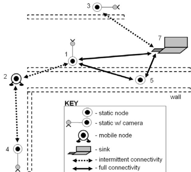
Fig. 6. Topology for Experiment 2: Static sensors with mobile intermediate node. Static sensor node 4 sends images to sink node 7 through intermediate mobile node 2 and static node 1.
