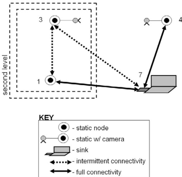
Fig. 5. Topology for Experiment 1: Static network. Sensor node 3 sends images to sink node 7 through intermediate node 1 when direct communication to the sink is unavailable.
