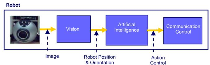
Fig. 3. Extended Small-Size robot architecture. Visual input from a camera mounted on the robot itself is processed by the Vision module to provide the AI module with robot positions and orientations. The AI module sends action command to the robot locally. Communication control is available for networking with other robots or a remote computer.
