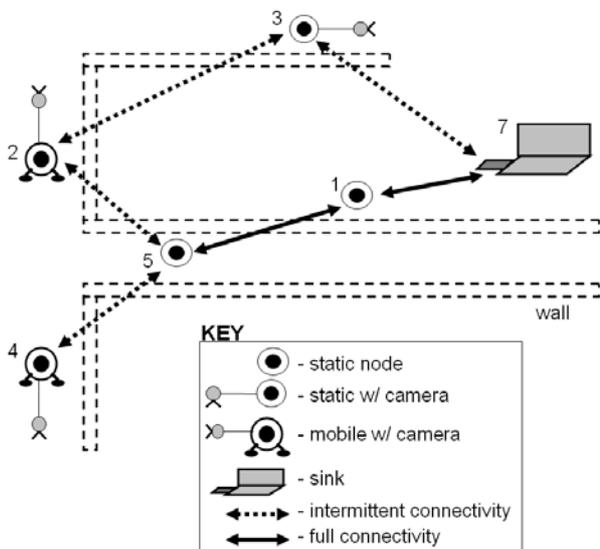
Fig 7. Topology for Experiment 3: Mobile sensors with static intermediate nodes. Mobile sensor nodes 2 and 4 send images to sink node 7 through intermediate static nodes 5 and 1.
