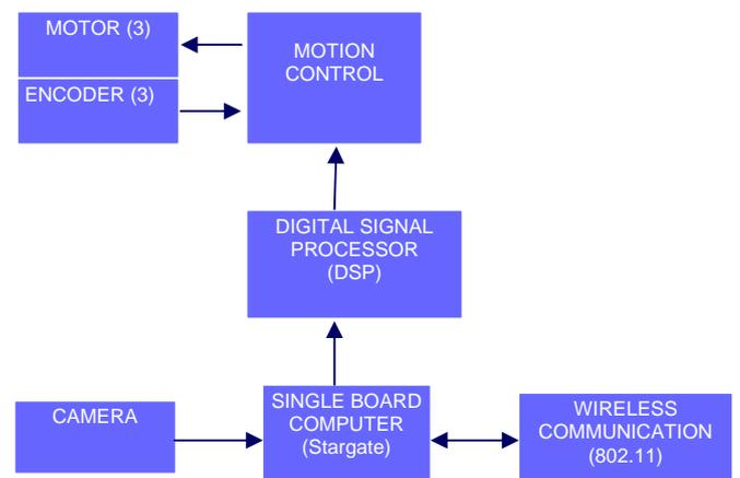
Fig. 4. Extended Small-Size robot block diagram. A DSP receiving remote signals via a wireless transceiver control three (or four) motors for omnidirectional movement. Additionally, the DSP control a dribbler and a kicker control mechanism.
