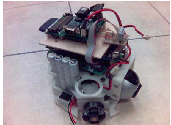
Fig. 2. Eagle Knights modified robot having local camera and 802.11 communication capabilities. The original robot architecture is maintained although replacing the transceiver with a direct linkage to the Crossbow Stargate (on top) managing wireless communication and local vision. Note how we replaced the kicker and dribbler with the camera due to camera.
