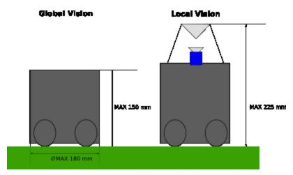
Figure 3: The maximum robot dimensions
