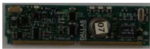
Figure 6: Dallas Semiconductors Tini Board (shown around two thirds actual size), with built in: processor, 1M memory and ethernet link.
