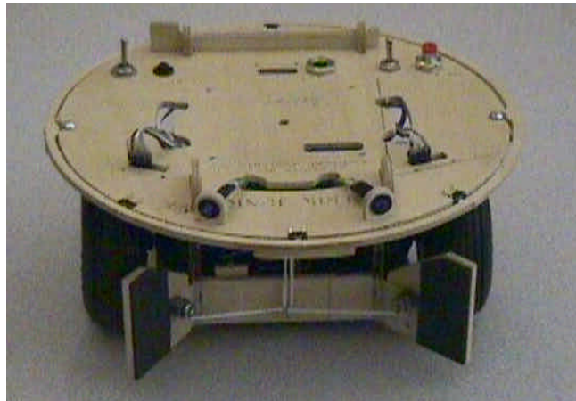
Figure 3.9. A TJ modified with a gripper. The design was developed by Jonathon Hurst, an undergraduate assistant on this project, in conjunction with the author. The gripper design and conversion process is located in Appendix A.
