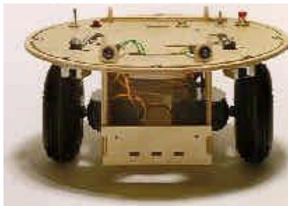
Figure 3.1. The Talrik Junior robot platform before modification.
