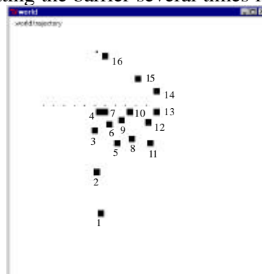
Figure 18. Rana Computatrix interacting with the 20 cm barrier before learning. The different dots correspond to the frog's trajectory from its initial location as it finally reaches the prey. We have added numbers corresponding to the frog's position in time. In this experiment the frog hits the barrier three times before perceiving the side of the barrier.
