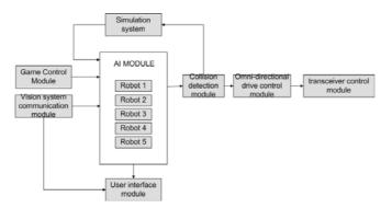
Fig. 4. Artificial Intelligence System Architecture.
