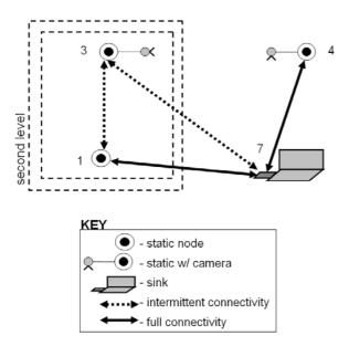
Fig. 5. Topology for Experiment 1: Static network. Sensor node 3 sends images to sink node 7 through intermediate node 1 when direct communication to the sink is unavailable.
