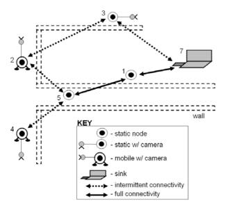
Fig 7. Topology for Experiment 3: Mobile sensors with static intermediate nodes. Mobile sensor nodes 2 and 4 send images to sink node 7 through intermediate static nodes 5 and 1.
