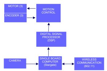
Fig. 4. Extended Small-Size robot block diagram. A DSP receiving remote signals via a wireless transceiver control three (or four) motors for omnidirectional movement. Additionally, the DSP control a dribbler and a kicker control mechanism.
