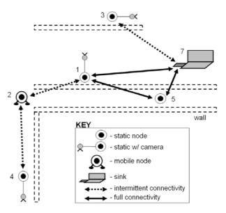
Fig 6. Topology for Experiment 2: Static sensors with mobile intermediate node. Static sensor node 4 sends images to sink node 7 through intermediate mobile node 2 and static node 1.
