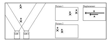
Fig. 1: Stereo vision with two parallel cameras
