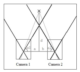
Fig. 2: Stereo vision object distance computation
