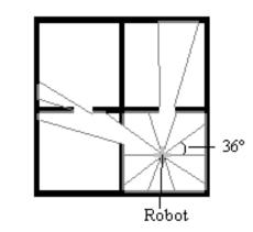
Fig. 9: What the robot at best can see
