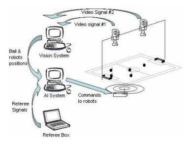
Fig 1. Typical architecture of a SSL team.
