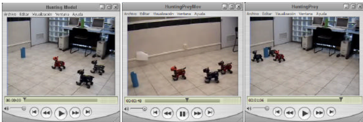
Figure 31. Left: Alpha wolf in red and beta wolves in dark blue. Robots pursue the blue colored cylinder corresponding to prey. Beta wolves keep a formation behind their leader. Center: Prey is manually moved with pack tracking it. Beta wolves maintain a formation behind their leader. Right: Eventually the robots get close to the prey attacking it by a surrounding motion.
