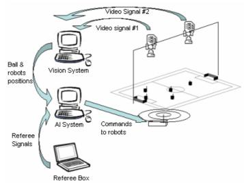
Fig 1. ITAM's RoboCup Small-Size league system architecture
