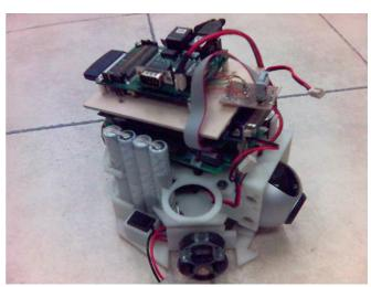
Fig 7. Eagle Knights modified robot having local camera and WiFi communication circuitry
