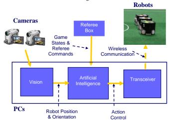
Fig 2. ITAM's RoboCup Small-Size league block diagram
