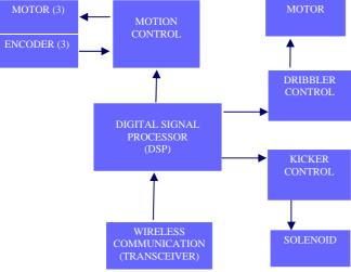
Fig 6. Eagle Knights robot block diagram
