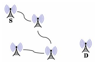
Fig 8. An example network in which there is no route from S to D. Existing on-demand routing protocols fail to deliver messages when a route cannot be established. StAR will buffer data at the node nearest to the destination until a route is available.
