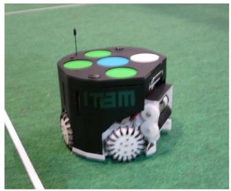
Fig 3. Eagle Knights robot showing colored patches
