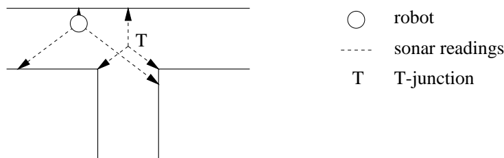
Figure 12: How the robot NX reaches and recognizes a T-section in a maze. The T-section is characterized by location T, which is defined as the location from where the three sonar readings are equal.
