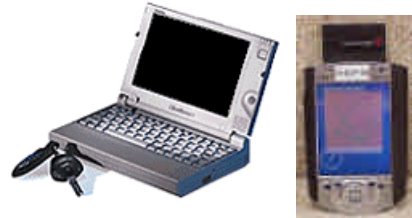
Figure 5 Toshiba Libretto sub-notebook and Compaq iPAQ Pocket PC with wireless network interface card.
