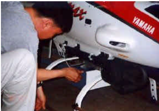
Figure 9. Mounting node in payload box onto the helicopter.
