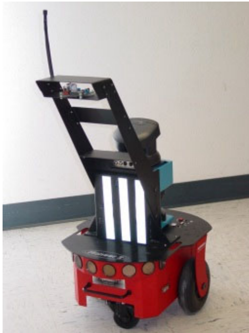
Figure 5. A Pioneer robot with laser-retroreflective tape attached to the back. This unit's beacon ID is 21 (10101 2 ).
