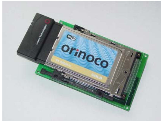
Figure 4. Top side of the Compact Ad Hoc Networking Radio, showing the Wavelan PC Card.
