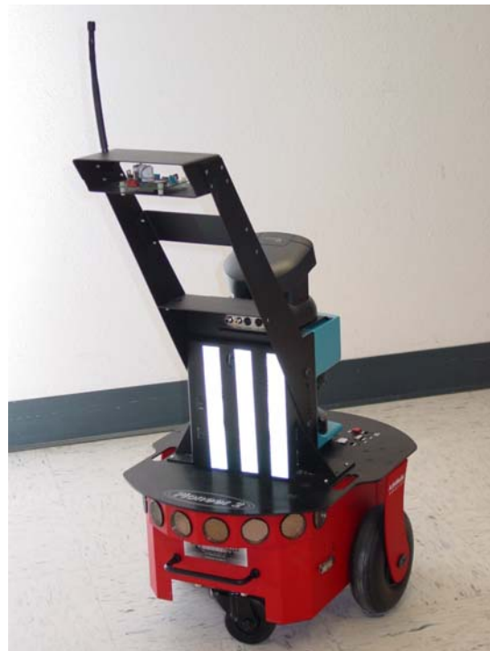
Figure 8. A relay robot with a retroreflective beacon on the back. This unit's beacon ID is 21 (10101 2 ).
