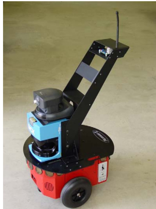
Figure 2. A Pioneer robot configured for communications relay and rearguard functions.
