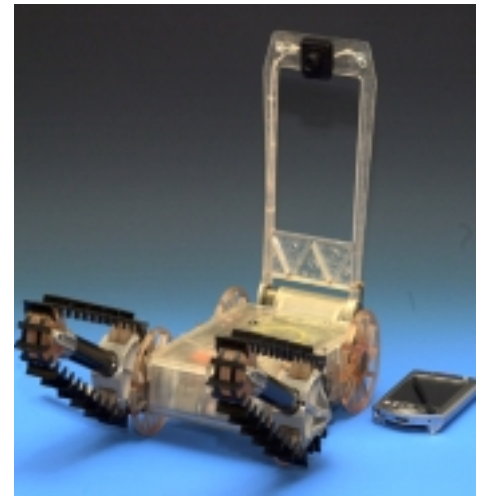
The HP iPAQ handheld and the Micro-Robot communicate over a wireless link to a PDA. The user can view camera images and control the robot remotely. Future versions will have autonomous guidance, navigation, and control.
