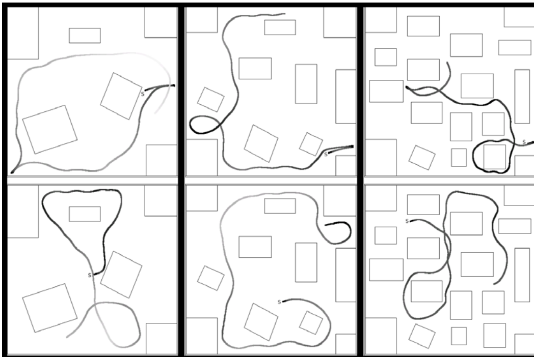
Fig. 8. Two specific trajectories among one hundred are illustrated in each environment, S being the starting position. The helicopter is able to make U-turns and to escape from dead-ends. As the grey-level of the trajectories shown is proportional to the current speed, they demonstrate that the helicopter slows down in cluttered regions and speeds up in open spaces.
